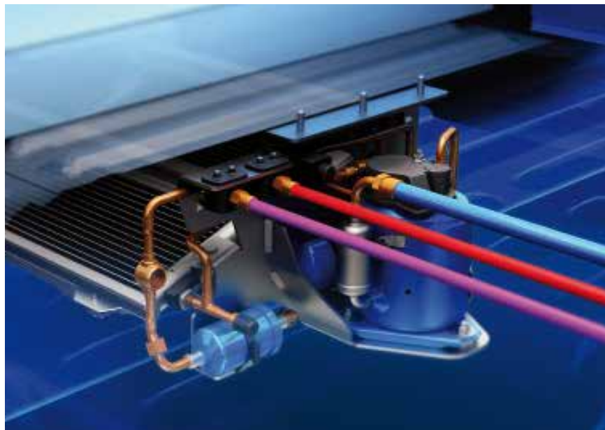
Condenser and compressor built in under chassis
