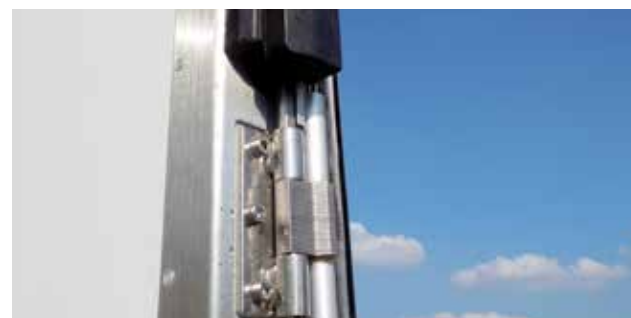
Automatically adjusting double-action spring door hinges
