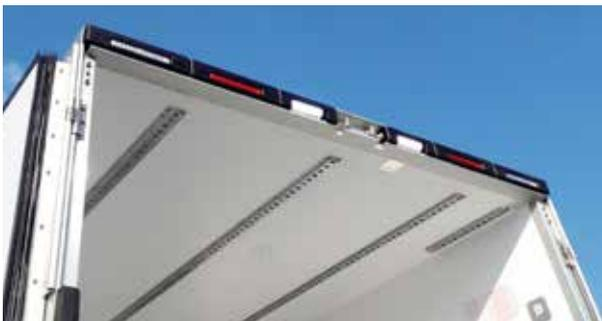
Optimised aerodynamics with a smooth rear, and front Cx Profiles
