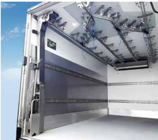
Distributing meat in sides requires specialized assisted unloading tools in order for the driver to handle the job safely. BEEFLIFT is a genuine “Cobot” that replaces the ladder technique: this controlled hydraulic arm provides effortless unloading of 250 to 500 kg carcasses.
