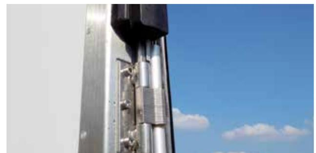
Automatically adjusting double-action spring door hinges
