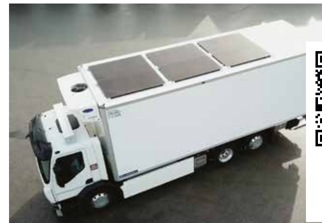
Lamberet has fitted the body roof with 6 solar panels giving a surface area of 10 m 2 providing peak power of 2400 W.
