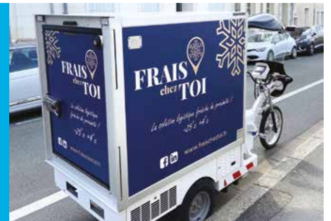
KLEUSTER Freegone is fitted with the new Frigoline body cell with coefficient K 0.31 and positive cold plug & play cooling unit.
