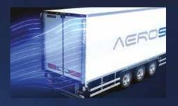
These aerodynamic spoilers effectively reduce fuel consumption, saving up to 1%. They innovate with automated deployment and retraction mechanism, fully transparent for the driver.
