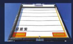
This new 100% Lamberet roller-shutter door, featuring an exclusive pneumatic mechanism, opens up new horizons in distribution: it combines the best useful-height/overall-height ratio, the widest passageway on the market with 2.42 m, and the first insulated curtain developed for frozen temperatures applications.
