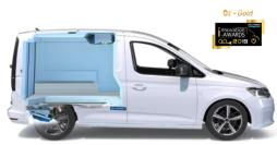
Kerstner e-Cooljet 106 unit integrated under the chassis
