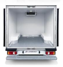
This body is intended for transport under controlled temperatures, in compliance with the ATP regulations in force.
