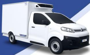
This body is intended for transport under controlled temperatures, in compliance with the ATP regulations in force.
