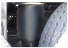
Reinforced 360 mm pneumatic suspension cushions: With an additional 44% of supporting surface, the load is better compensated, the suspension sags less and offers greater résistance, reducing the shifting of the centre of gravity. A double pneumatic circuit independently feeds each side of the suspension in order to dampen rolling when taking bends.
