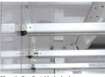
22 vertically adjustable duplex beams every 25 mm which are also removable: Each with a capacity of 1 tonne, enabling a load of 33 800x1200 mm pallets to be modulated. Intermediate rails can be installed for 800x600mm pallets.
