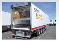
Rising opening: The insulating curtain frame, with manual or electric silent opening (PIEK certificate 54 dB), facilitates distribution. Ultra-resistant, in stainless steel, fully bolted, with complete protection (sill, vertical upper and lower posts).
