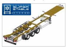
SuperStable chassis: A completely new feature, combining the control of the centre of gravity, with H-spars in THLE steel with a reduced height of 180 mm, and an enlarged running gear which reduces sagging during cornering, to minimise the critical speed factor when cornering.
