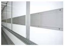
100% recessed vertical duplex rails: The duplex system consists of 12 high performance antiabrasion aluminium rails, aligned with a centre distance of 1208mm, without any rebound onto the side walls. The quality of insulation has been 'reinforced' without compromising the net width or handling during loading operations.
