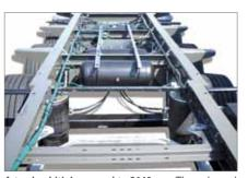
A track width increased to 2140mm: The enlarged running gear is a completely new feature. The centre distance between the spars in the central module is increased by 100mm to 1400mm, bringing the track width to 2140mm, which is the most demanding stability standard for tankers. The Super Stable chassis increases the tipping threshold by 15%: a gain calcualted in accordance with EEC regulation No. 111, appendix 4.
