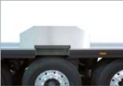
**4 reinforced handling zones:** lower handling profiles intended for grab cranes, and lateral protective plates, for transfer of the SR2 Rail-Road units onto rail cars in complete safety.
