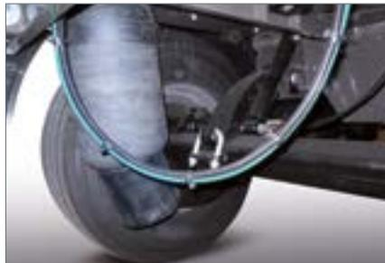
**Duplicated suspension cushions:** the 6 doubled suspension cushions are fully adapted for transshipment on rail car platforms, without travel limitation.
