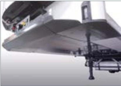
**Enlarged front plates:** maximum protection for more robust use by third parties during repeated transshipment operations. The front face is thus preserved from impacts on its entire width.
