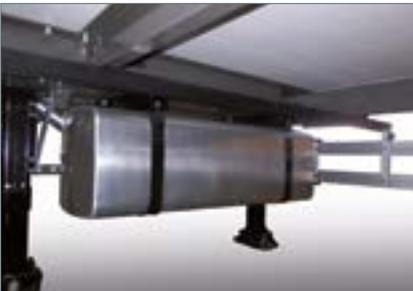
**Maximum autonomy:** large capacity 420 litre aluminium container. Resistant to age hardening and corrosion, its exceptional capacity is combined with the performance of the Lamberet composite insulation to offer enhanced autonomy. A real advantage for long-distance rail transport.
