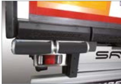
**Integrated protection system:** the exclusive Lamberet design means that the rail transport dimensions are compliant with reinforced protection at the rear of the chassis, equipped with double horizontal buffers with shock-absorbing rollers. The vertical sections and sill are totally protected by integrated buffers.
