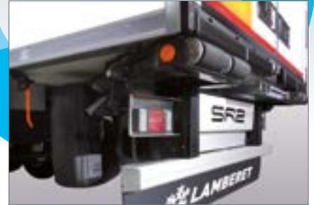
**Re-dimensioned rear module:** with a 300 mm contraction of the rear module equipment, positioning of the SR2 Rail-Road unit on the rail car is facilitated without the risk of damage.
