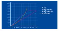
Less traction force: Lower consumption, less CO2: The reduced scuffing and X-City's ability to achieve an optimal turning circle relative to the tractor significantly lowers the traction force needed during turns, by up to 66%. The result is 12% lower consumption in a city environment. As a second benefit, the tractor's power can be reduced.
