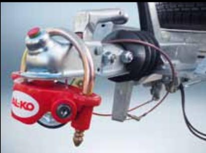
**Anti-theft lock (optional):** For heightened security, this dedicated lock fastens onto the drawbar, thereby preventing anyone from towing away your trailer. Ceiling light (not depicted): If the body is equipped with a cooling unit, a ceiling light illuminates the loading area.
