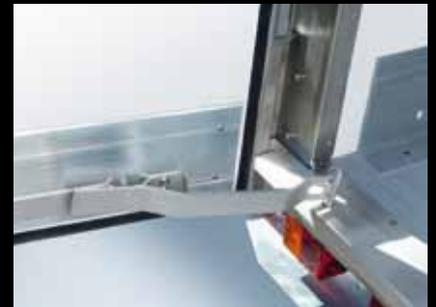
**Door retainer:** Lamberet trailers have a door retainer (made of rubber or T-shaped, depending on the model). To facilitate operations in narrow parking areas, 180° retainers are optionally available (see photo).
