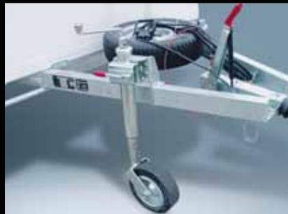
**Body fittings (standard):** All trailers are equipped with a full set of fittings: A jockey wheel to facilitate turning; two stabilizing stands at the rear and a parking brake for static usage or parking; a spare wheel and crank; a 13-pin trailer plug with removable 7-pin adapter.
