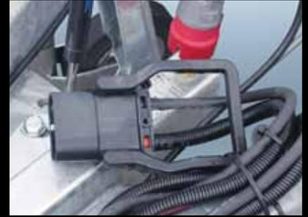
**Vehicle connection (road mode):** In road mode (optional), the electrical unit is connected by means of a "fenwick" plug to the pulling vehicle's battery, whose alternator must have at least 90 A. Below that, a "power kit" installed post-sales is adaptable to some vehicles.
