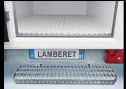
**Footstep:** Built into the 750 kg version or attached onto the 1300 or 2000 kg version, the fixed steel "one-level" no-slip foot-step makes it easier to access the loading area.
