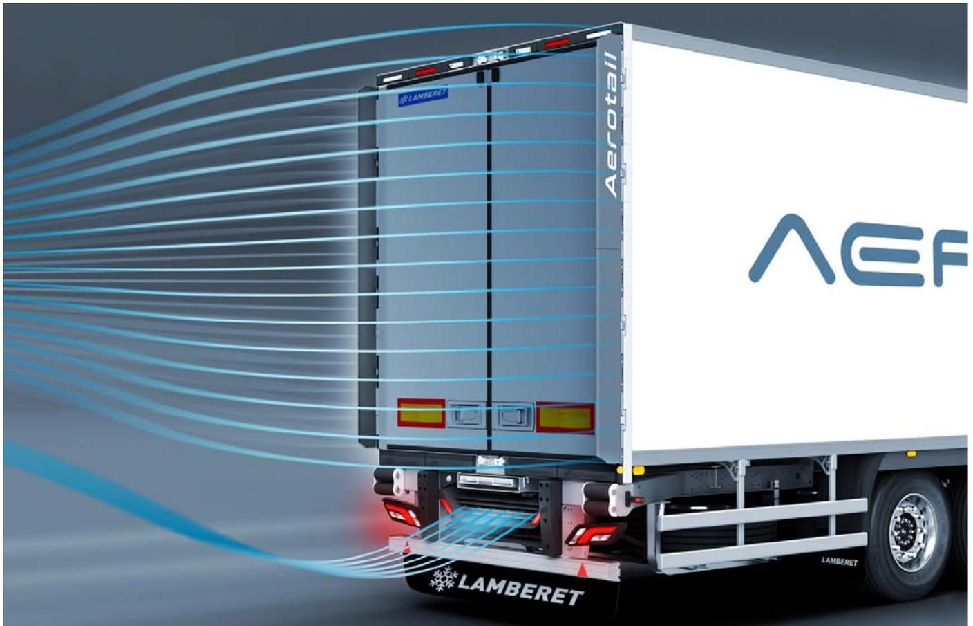
*Aerotails are the first rear spoilers that are fully automatic.
