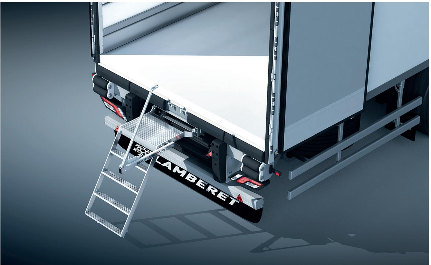
The SAFESTAIR integral handrail automatically deploys when taking out the ladder.
