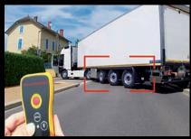
Remote control for the steering axles.
