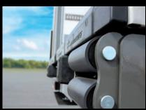
Anti-shock protection and steel twin tube roller buffers (Lamberet patent). Impacts are absorbed by the roller buffers fitted with an external steel tube and cellular rubber inside, mounted on a steel axis. Residual efforts are dissipated by the high inertia reinforcement arms on the chassis.
