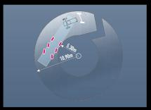
A turning circle reduced by 30%. The SR2 SuperCity has the benefit of the maximum capacity of a refrigerated fixed triaxle semi-trailer with a 7450 wheelbase, but its turning circle has been reduced from 6873 mm to just 5016 mm. This is less than a 21 pallet carrier (5600 mm)!
