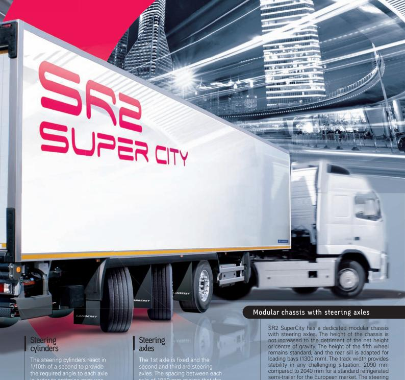
The steering cylinders react in 1/10th of a second to provide the required angle to each axle in order to optimise manures. They are fitted with a centrally controlled greasing system for ease of maintenance. An independent battery pack smooths out peaks in demand in situations of high levels of demand so that an immediate response is always guaranteed. The 1st axle is fixed and the second and third are steering axles. The spacing between each axle of 1850 mm means that the
