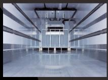
Anti-slip «floating» PIEK aluminium floor (55 dB). A Lamberet patent, combining resistance with wear and sound insulation. Its profiles incorporate longitudinal anti-slip grooving. A peripheral joint delinks the sound bridge.
