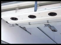
Silent multi-temperature refrigeration unit (PIEK). The SuperCity chassis has a sufficiently wide wheelbase to accommodate silent multi-temperature refrigeration systems such as the CARRIER Vector City 1850 MT City unit. The unit's motor and exhaust are located under the chassis which minimises sound emissions.
