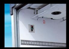
100% pneumatic autonomous raising and lowering with internal controls. An exclusive LAMBERET - HALDEX feature, controls the raising and lowering valve from an additional air reserve (60 litres). It has non-coupled functioning without electrical power. The internal controls enable levelling of the SR2 SuperCity.
