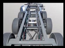
Flared chassis module with steering axles. The modular design of the SR2 chassis means that the steering axle system can be accommodated without increasing the height of the chassis.
