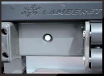
TOTALLY integrated Soft-Docking. When approaching the loading bay, 2 radars integrated and protected inside the end of chassis frame crossmember detect its presence and apply the brakes on the trailer automatically and progressively before impact. Your capital investment is protected from violent impacts. Drivers are relieved of the stress of potential damage even in poor visibility or complicated manoeuvres, as can be frequent in towns.
