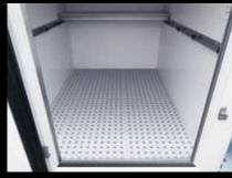
Grating (optional): The floor is covered with removable, slatted plastic slabs, which are easy to wash, in order to allow optimized ventilation, prevent contact between food items and the ground, and protect the cargo from condensation moisture. Recommended for the HACCP hygiene approach.
