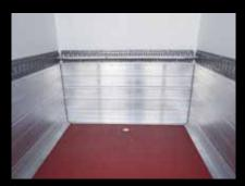
Securing rails and runners (optional): The aluminum runners protect the walls from repeat impacts. The securing rails secure and stabilize your goods during transport.
