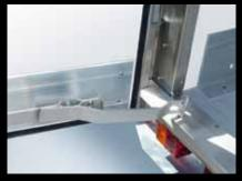
Door retainer: Lamberet trailers have a door retainer (made of rubber or T-shaped, depending on the model). To facilitate operations in narrow parking areas, 180° retainers are optionally available (see photo).
