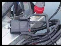
Vehicle connection (road mode): In road mode (optional), the electrical unit is connected by means of a "fenwick" plug to the pulling vehicle's battery, whose alternator must have at least 90 A. Below that, a "power kit" installed post-sales is adaptable to some vehicles.
