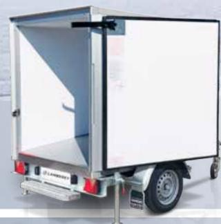
Professional quality accessible with a B\* or B96\* permit! This assembly combines an isothermal or refrigerated body of very high quality, with a robust, stable single-axle chassis. Ideal equipment for transportation or as a cold room with occasional boosts.
