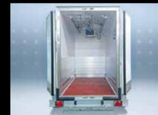
**Meat hooks (optional):** In the meat transport version, trailers of 1300 kg and above have inserts in the roof for fastening the right system for your business: Fixed or removable hook bars, slider-type hangers, bi-rails, tubes, or a hybrid. Additionally, the floor can be red-tinted, no-slip treated coarse-grained steel, (specific).
