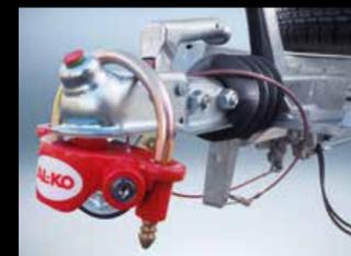
**Anti-theft lock (specific option):** For heightened security, this dedicated lock fastens onto the drawbar, thereby preventing anyone from towing away your trailer. Ceiling light (not depicted): If the body is equipped with a cooling unit supplied by Lamberet, a ceiling light illuminates the loading area.
