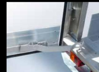
**Door retainer:** Lamberet trailers have a door retainer (made of rubber or T-shaped, depending on the model). To facilitate operations in narrow parking areas, 100° retainers on OT2 are optionally available (see photo).
