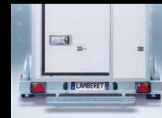
**Footstep:** Built into the 750 kg version or attached onto the 1300 or 2000 kg version, the fixed steel "one-level" no-slip foot-step makes it easier to access the loading area.
