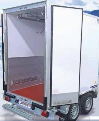
Offering 5 to 7 m<sup>3</sup> of useful volume, this is a true customizable vehicle based on your activity and suited to the transport of large-volume perishable foodstuffs. In its "meat door" version with full rear opening, meat hooks, extra useful height, and red-tinted no-slip floor, this is the ideal solution for meat industry professionals.
