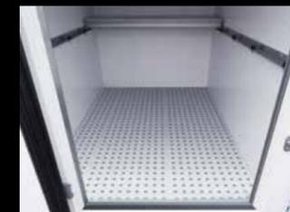
**Grating (optional):** The floor is covered with removable, slatted plastic slabs, which are easy to wash, in order to allow optimized ventilation, prevent contact between food items and the ground, and protect the cargo from condensation moisture. Recommended for the HACCP hygiene approach.
