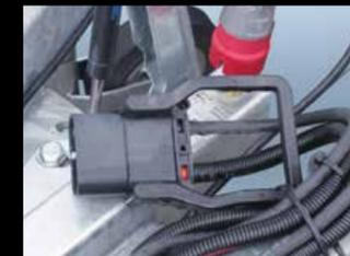
**Vehicle connection (road mode):** In road mode (optional), the electrical unit is connected by means of a "fernwick" plug to the pulling vehicle's battery, whose alternator must have at least 90 A.
