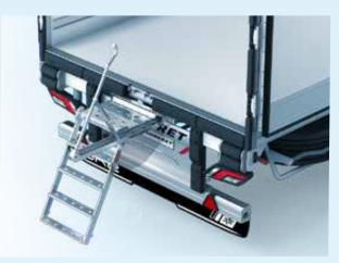
Secure rear access with automatic handling ramp
