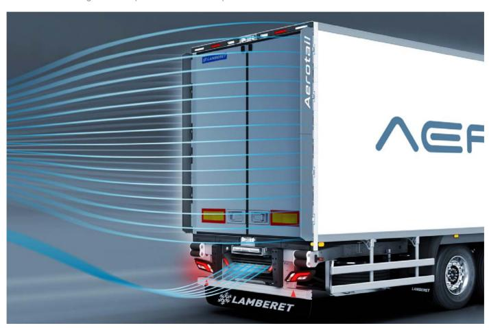
Aerotails are the first rear spoilers that are fully automatic. The observed consumption saving is a minimum of 1% in mixed conditions.
